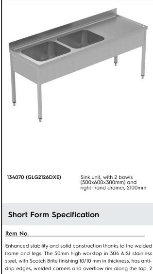
drip edges, welded corners and overflow rim along the top. 2 welded and polish sink bowls in 304 AISI stainless steel supplied with overflow pipe and 2" drain hole. Upstand h=100mm with 10mm radius corner covered on the back with AISI 304 stainless steel spot welded profile. Square section legs and height adjustable feet (-20/+30 mm) in 304 AISI stainless steel.
